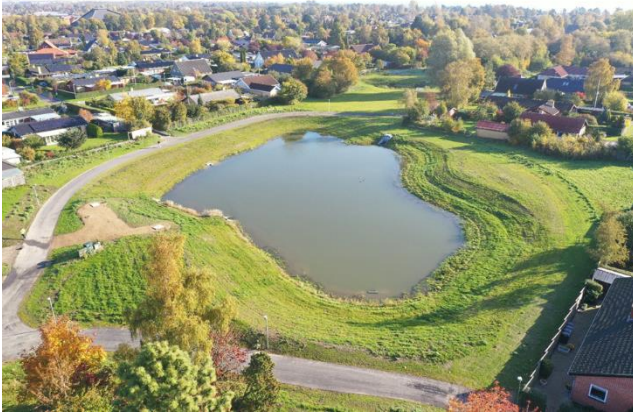
Figure 42 One of several retention systems, included in the climate adaptation plan for Birkedalen
